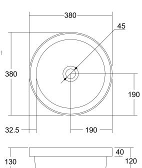
Dimensions are shown in millimetres. Due to the handcrafted nature of Omvivo products measurements are subject to a  $\pm$ -5mm manufacturing tolerance.
